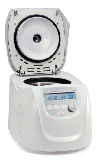
SHCHEER hematocrit centrifuge with AC24P hematocrit rotor is used for determination of volume fractions of erythrocytes in blood for diagnostic purposes and doping tests. Also it is used for the photometric determination of bilirubin content in neonate blood samples. Hematocrit centrifuge with A24-2P tube rotor, can be used for extraction of DNA and RNA.
